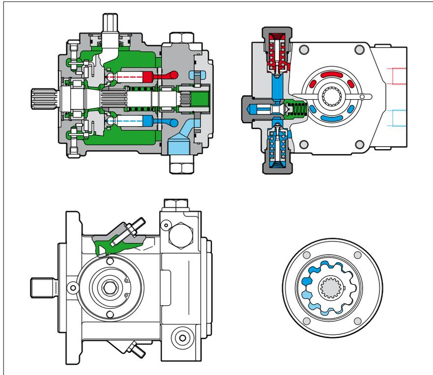
Fig. 3: Cut-away view of A10VG with mechanical trunnion adjustment
