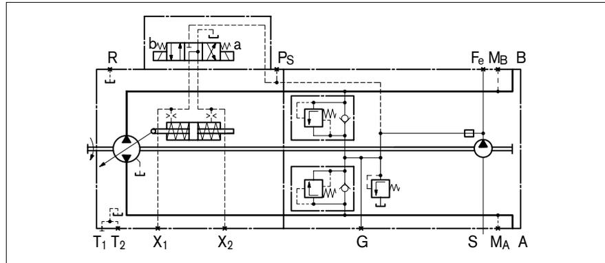
**Fig. 14: Hydraulic circuit diagram of A10VG with electric two-point control, with switching solenoid**
