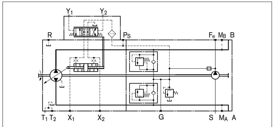
Fig. 6: Hydraulic circuit diagram of A10VG with hydraulic control, pilot-pressure related
