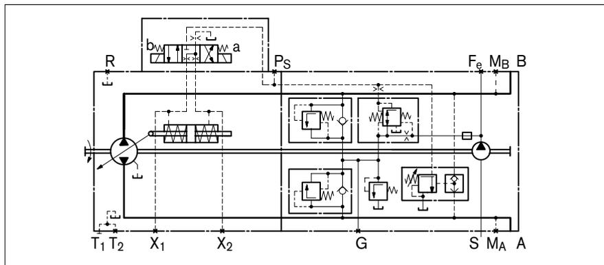
Fig. 11: Hydraulic circuit diagram of A10VG with automatic control, hydraulic, speed related
