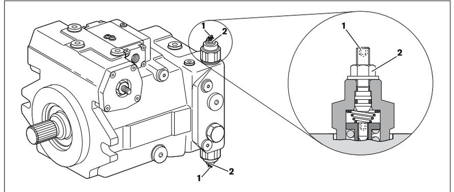
Fig. 15: Activating the bypass function
