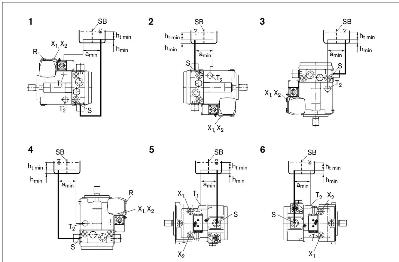
Fig. 20: Below-tank installation with installation positions 1-6
