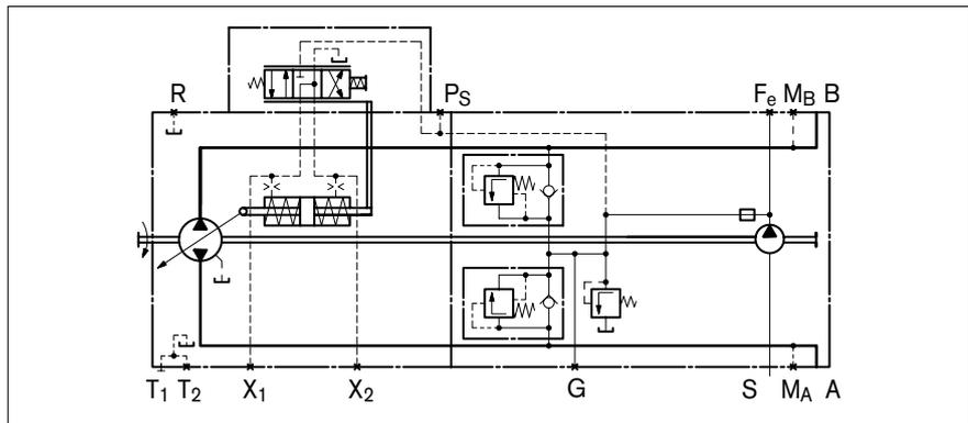
Fig. 8: Hydraulic circuit diagram of A10VG with hydraulic proportional control
