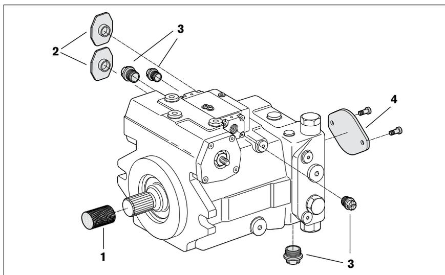
**Fig. 23: Removing transport protection**
