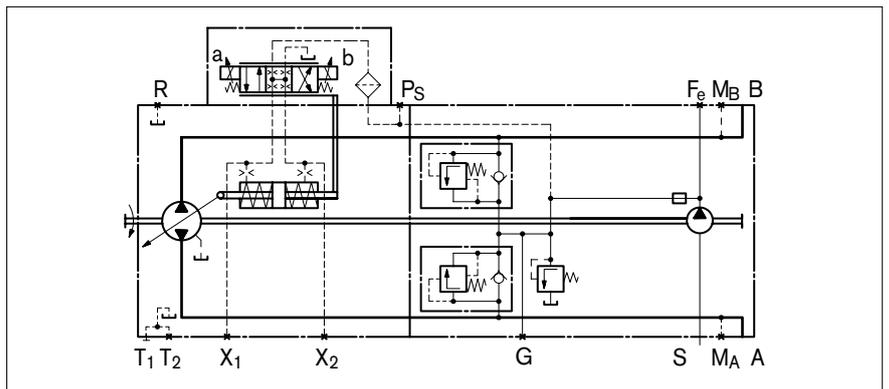
Fig. 13: Hydraulic circuit diagram of A10VG with electric proportional control
