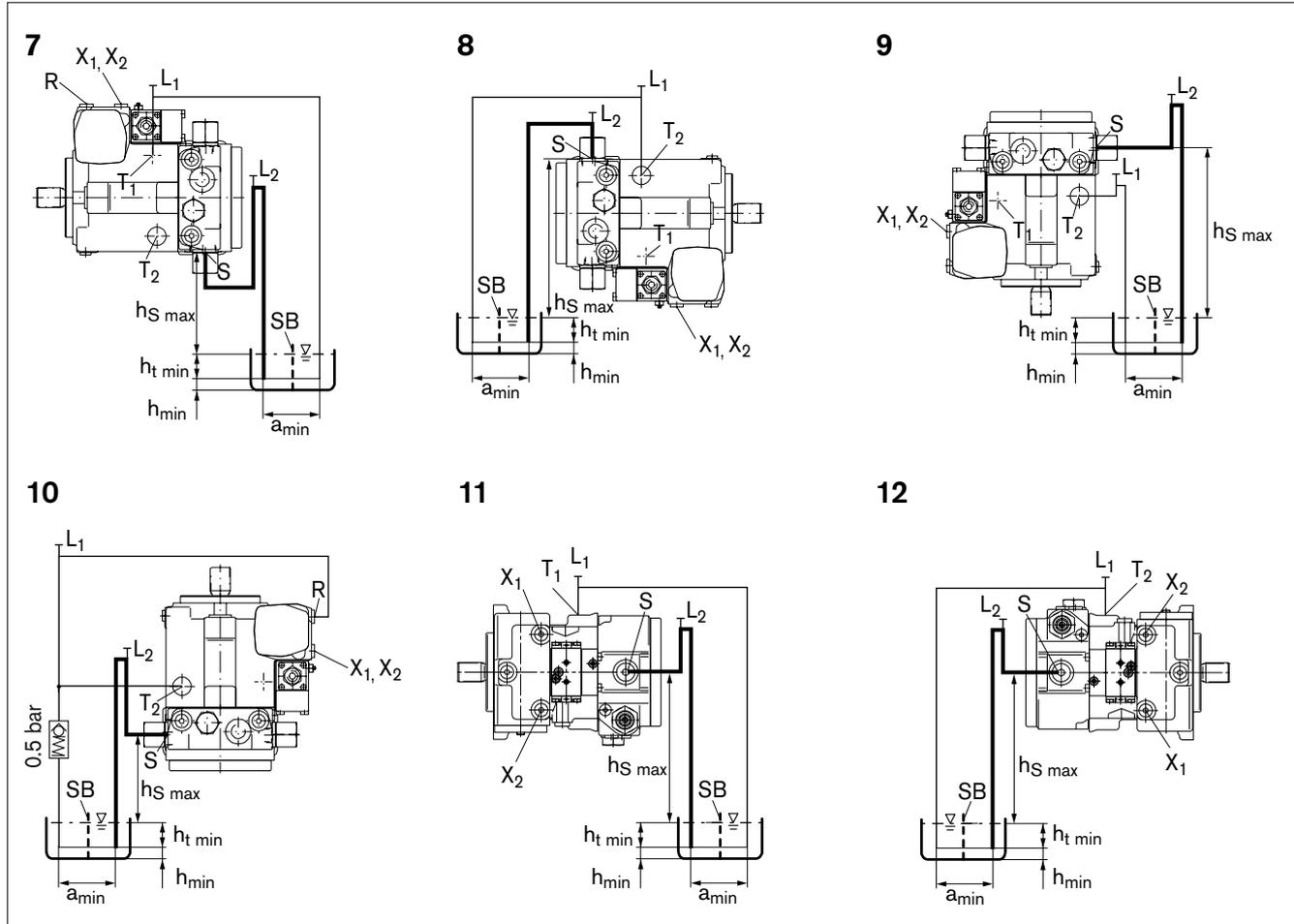
Fig. 21: Above-tank installation with installation positions 7–12
