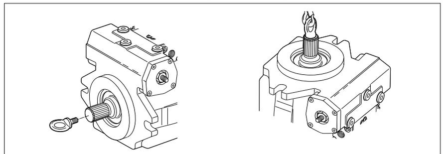
**Fig. 17: Fixing the ring screw**
