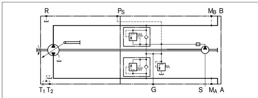
Fig. 4: Hydraulic circuit diagram of A10VG with mechanical trunnion adjustment
